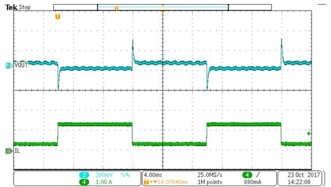
Figure 20. Load Transient
