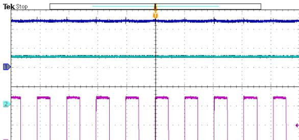
Figure 12. SCT2320 Switching Node Waveform
