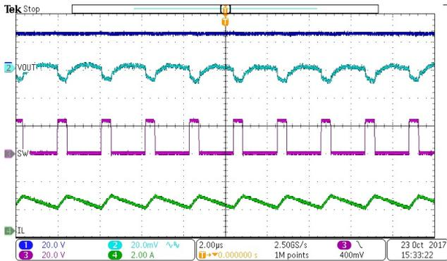
Figure 15. SW node waveform and Output Ripple
